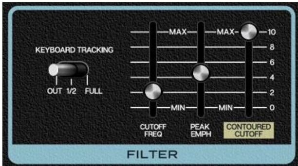
The Filter section is a 24 db/oct lowpass filter that removes high frequencies as its cutoff frequency setting is decreased from max, resulting in a dulling of sound. This is a version of the classic transistor "ladder" filter, famously heard in the Moog Minimoog synthesizer, and renowned for its meaty, fat sound.
